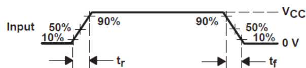
Figure 6-5. Voltage Waveform Input Rise and Fall Times
